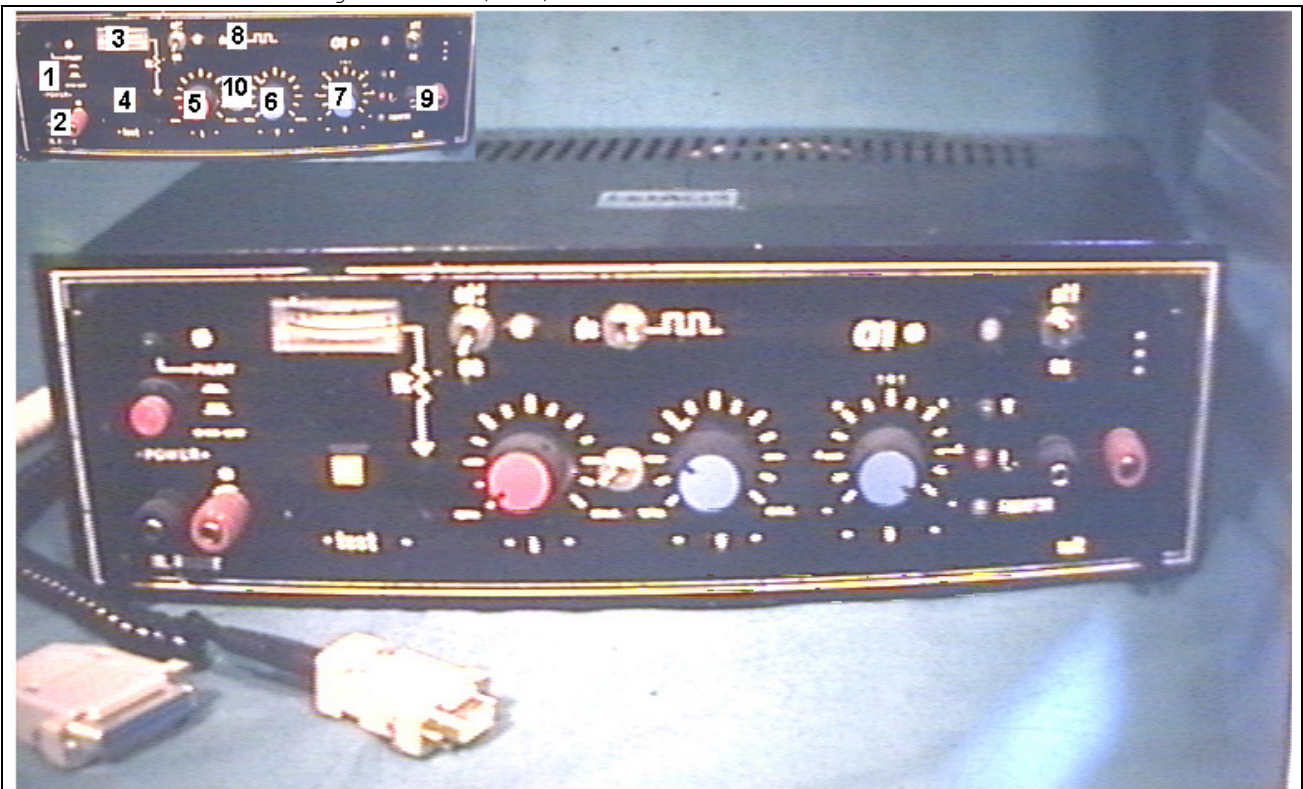
Computer driven electro therapy device. 1, Power on; 2, Constant current output; 3, current checker; 4, push button to check actual current level; 5, current
